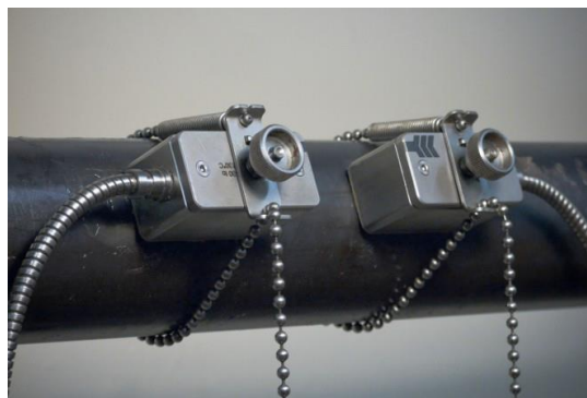
Illustration 5: Sensor mounting with clips and chains
